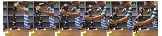
Fig. 3: Kinesthetic demonstration of reaching to an object (yellow box). Captured task-space pose of the end-effector is used as input.
